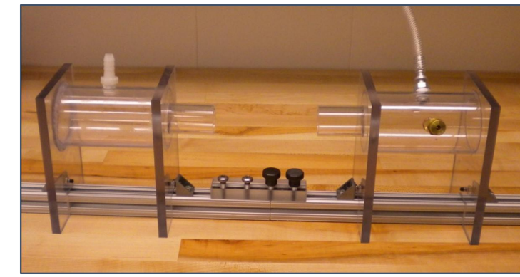
Figure 2: Negative pressure airway system for modeling the collapsibility of the human airway in sleep apnea
