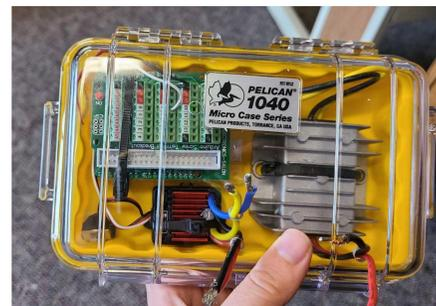
In 2020 the GBG! MKE team started to offer an acceleration controller microprocessor system for self-steer vehicles. This system was designed to slowly ramp the speed of the car up from zero to full power. This ramp-up is much slower than the car's internal systems and was designed to address startle reactions resulting from initial car start-up.
