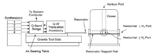
Figure 1. Overall assembly of the W-band spectrometer
