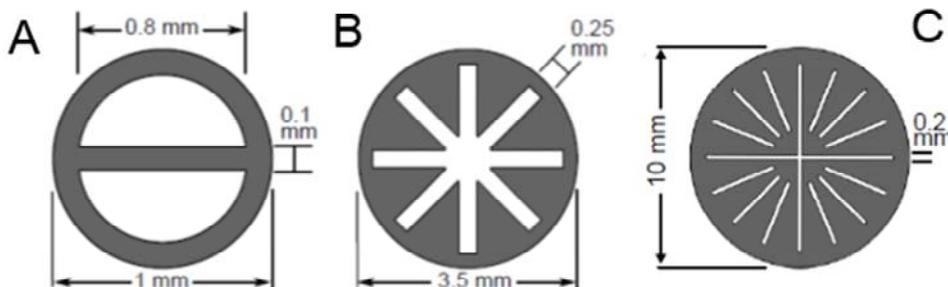
**Figure 1.** Illustration of the three new sample holder geometries: A) DoubleDee, B) AquaStar, and C) AquaSun
