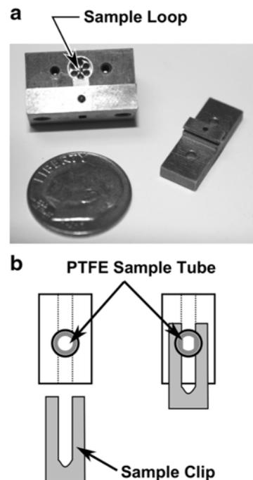
**Fig. 1.** a) New Seven-Loop–Six-Gap LGR resonator with gas exchange port and sample holder. Highlighted here is the sample loop 0.825 mm ID, located in the center of the Seven-Loop–Six-Gap geometry. b) New sample holding mechanism for PTFE samples uses a clip that compresses the sample tube and holds it in place.
