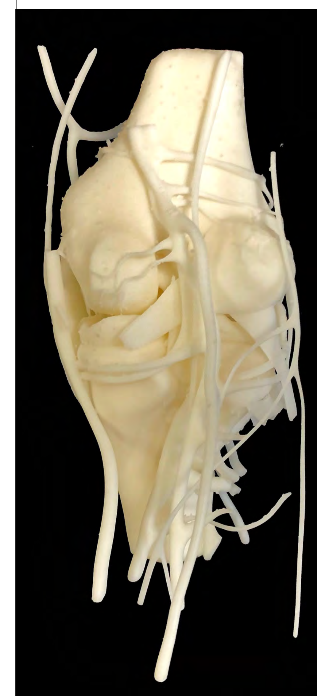
Figure 8: Posterior view of 3D printed knee joint (bones, connective tissue, arterial and venous systems, nerves) in Formlabs White V4 Resin.
