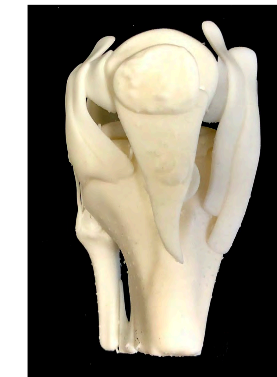
Figure 9: Anterior view of tibial segment of knee joint (bones and connective tissue) in Formlabs White V4 Resin.
