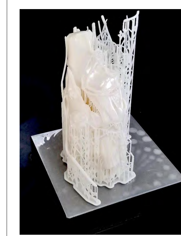
Figure 4: Arterial system surrounding the knee joint printed in Elastic 50A Resin.
