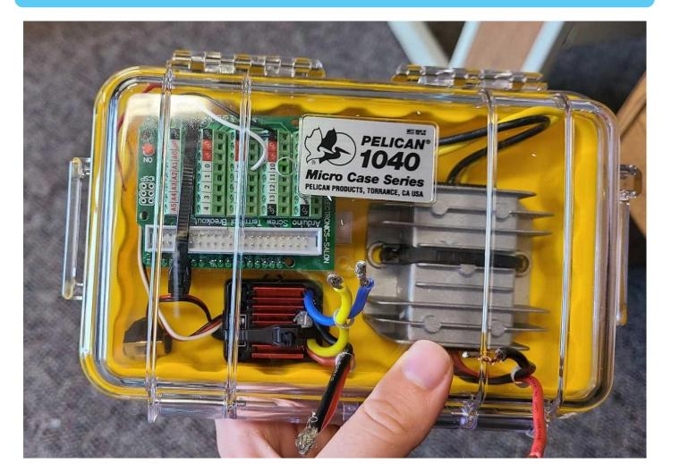
In 2020 the GBG! MKE team started to offer an acceleration controller microprocessor system for self-steer vehicles. This system was designed to slowly ramp the speed of the car up from zero to full power. This ramp-up is much slower than the car's internal systems and was designed to address startle reactions resulting from initial car startup.
