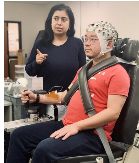
Priya Balasubramanian conducts an experiment in which brain signals are measured while the volunteer contracts their wrist to fatigue.
