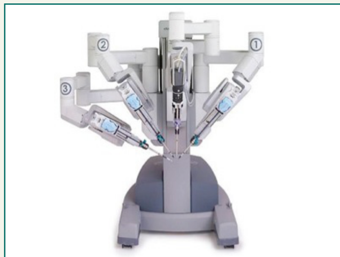
Figure 2: da Vinci Si robot system currently used at The Medical College of Wisconsin
