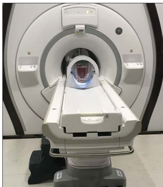
Figure 3. 7T MRI Scanner on the MCW campus actively imaging a rectal cancer specimen.
